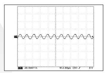
Figure 16: Output voltage ripple, Vout, at nominal input voltage and rated load current (20mV/div). Load capacitance: 1µF ceramic capacitor and 10µF tantalum capacitor. Bandwidth: 10MHz. See Figure 14.
