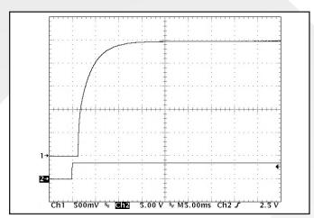
Figure 9: Turn-on transient at full resistive load and zero output capacitance initiated by ENA2. Input voltage pre-applied. Ch 1: Vout (500mV/div). Ch 2: ENA2 (5V/div).
