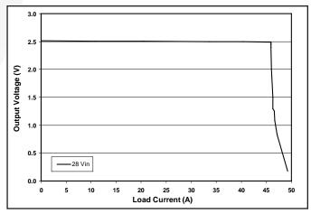
Figure 6: Output voltage vs. load current showing typical current limit curves.
