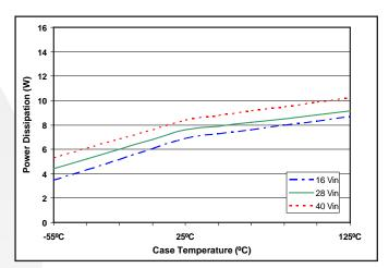
Figure 4: Power dissipation at nominal output voltage and 60% rated power vs. case temperature for input voltage of 16V, 28V, and 40V.
