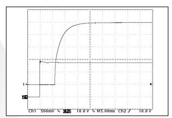
Figure 10: Turn-on transient at full resistive load and zero output capacitance initiated by Vin. ENA1 and ENA2 both previously high. Ch 1: Vout (500mV/div). Ch 2: Vin (10V/div).
