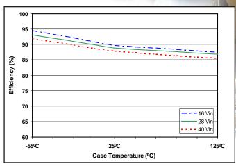
Figure 2: Efficiency at nominal output voltage and 60% rated power vs. case temperature for input voltage of 16V, 28V, and 40V.
