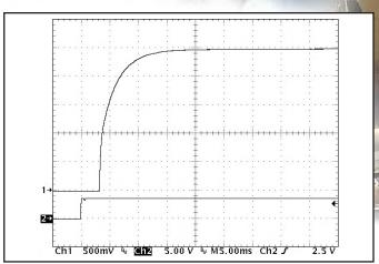
Figure 8: Turn-on transient at full resistive load and 10mF output capacitance initiated by ENA1. Input voltage pre-applied. Ch 1: Vout (500mV/div). Ch 2: ENA1 (5V/div).
