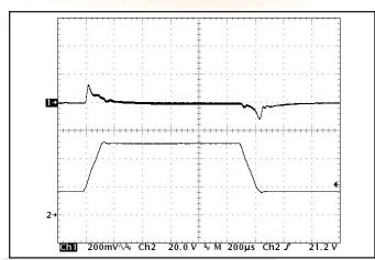
Figure 13: Output voltage response to step-change in input voltage (16V - 50V - 16V). Load cap:  $10\mu F$ ,  $100m\Omega$  ESR tantalum cap and  $1\mu F$  ceramic cap. Ch 1: Vout (200mV/div). Ch 2: Vin (20V/div).
