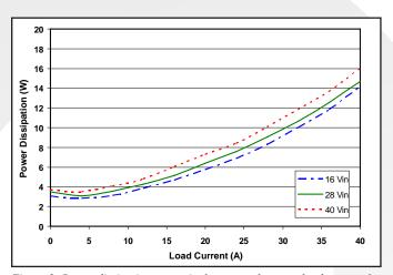
Figure 3: Power dissipation at nominal output voltage vs. load current for minimum, nominal, and maximum input voltage at Tcase=25°C.
